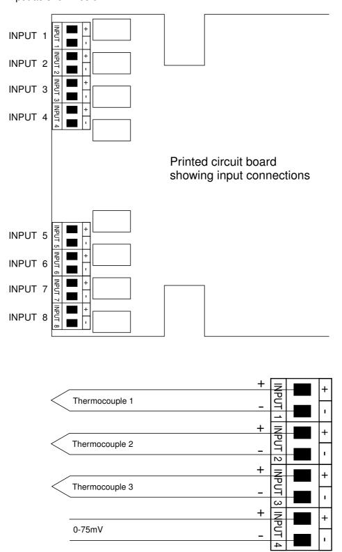
Example: 3 x thermocouples connected to inputs 1, 2, & 3. 0-75mV input on input channel 4.
