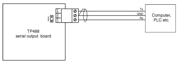
RS485 connections - use twisted pair shielded cable
