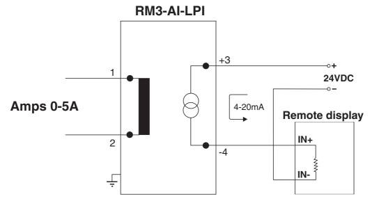
**Example 3** - connection to a remote display using the optional internal RM3-PS dual 24VDC output power supply to power the output loop.
