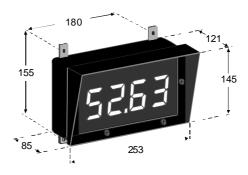
Four mounting kit brackets are supplied for use with all 100 & 200mm display models. Diagrams below illustrate vertical and horizontal installation. If mounting without the brackets is preferred then the 9mm dia. case holes provided for the brackets can be used as alternative mounting holes. If the brackets are not used in mounting these holes should be sealed against dust and water.
