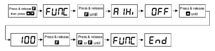
Example: Entering CRL mode to change decimal point dCPL function from 0 to 0.02
