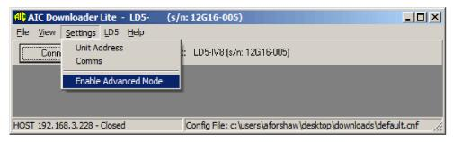
To enable advanced operations such as Calibration hold "Ctrl" then click on Settings then click on Enable Advanced Mode
